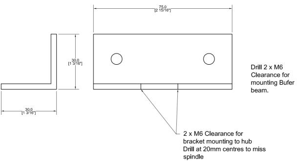
Sheet 5 Assembled Raising Block and Mounting Bracket
